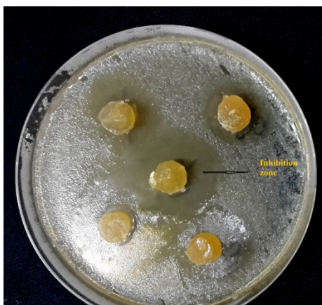
Figure (1): Cup assay method for detection colicinogenic E. coli
